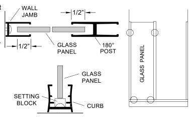
NOTE: To accommodate out of plumb walls, the 1/2" overlap may be adjusted 1/4" to 3/4"
