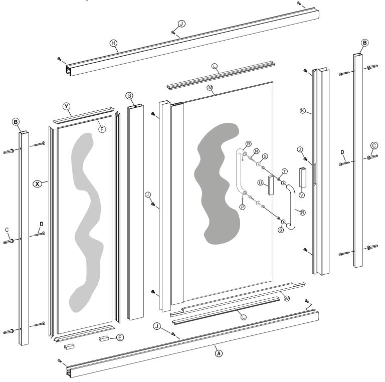
The shower door is completely reversible and can be installed hinge-left or hinge right.
