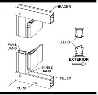
Pull the bottom end of the hinge jamb tight to the curb filler [\*R] and plumb the jamb. Drill two 1/8" holes thru the hinge jamb and into the wall jamb (or post) 3/8" to 3/4" from the wall and approximately 1/4" vertically from the ends of the jamb. Drill a third hole centered between the first two. Attach the hinge jamb/door panel permanently with three #6 x 3/8" truss head screws [\*C].
