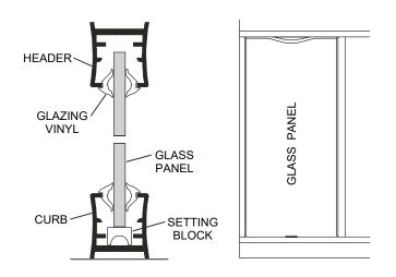
Using Onyx Adhesive / Sealer, caulk the entire exterior and interior of the shower door. Also, fill the small gaps at the corner of the vinyls that hold the glass side panels.
