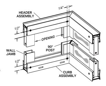
Press the hinge jamb/door panel assembly [\*A ] and strike jamb [\*B] (with magnetic strip) over the wall jamb and/or framing posts. Refer to Step #1 of the STIKSTIK instruction sheet for the proper handing of the door.
