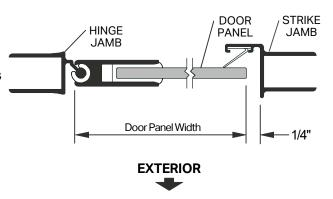
Snap both fillers\* [R] into the curb and header between the hinge and strike jambs with the raised edge to the exterior. Center the curb filler between the hinge and strike jamb (use masking tape to hold in position).
