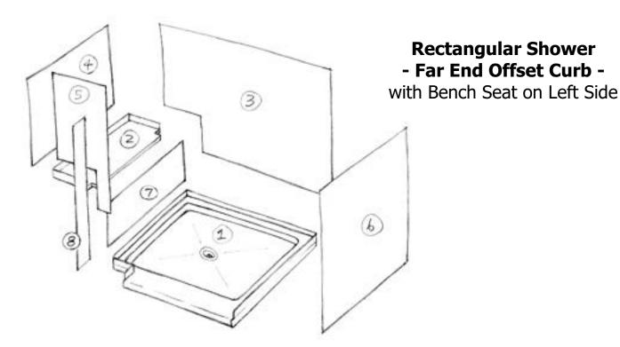
Copy this page, write your dimensions on the copy, and fax to us for a quote. **Always give stud-to-stud measurements for base, framing height of bench seat support structure, and distance to top of wall panels from the floor.** We will figure clearances etc.
