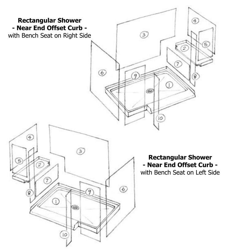
Copy this page, write your dimensions on the copy, and fax to us for a quote. **Always give stud-to-stud measurements for base, framing height of bench seat support structure, and distance to top of wall panels from the floor.** We will figure clearances etc.
