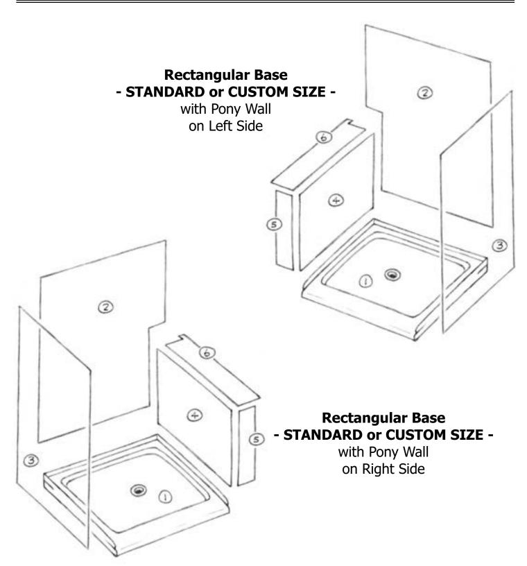
Copy this page, write your dimensions on the copy, and fax to us for a quote. **Always give stud-to-stud measurements for base, framing height of bench seat support structure, and distance to top of wall panels from the floor.** We will figure clearances etc.
