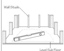
The Onyx base can be installed onto wood sub floors, concrete, underlayment board such as HardiBacker, tile, vinyl or other similar flooring materials.
