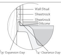
Walls should be plumb and framing should be completed before the shower base is installed.
